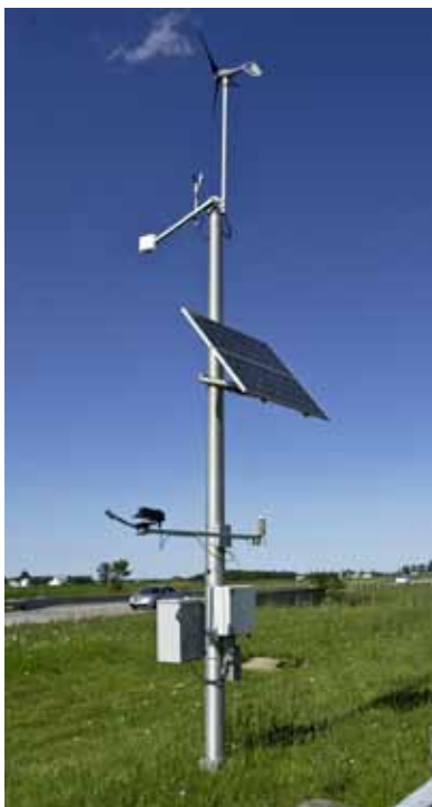
Vaisala Permanent Traffic Analyzers are installed with each RWIS wireless station. Photo courtesy of the Ohio Department of Transportation.
